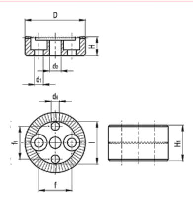
$$\begin{array}{lll} D & = 32 \\ d & = M6 \\ d1 & = 5.3 \\ d4 & H11 & = 5 \\ f & = 18 \\ f1 & = 18 \\ H & +/-0.9 & = 9.0 \\ H1 & = 18 \end{array}$$
